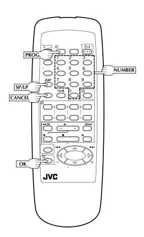
With G-CODE, timer programming is greatly simplified because each TV programme has a corresponding code number which your recorder is able to recognise.
